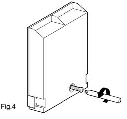
Prise cover loose using screwdriver in position (1) then lever off with screwdriver in position (2) at either side. See Fig. 5.
